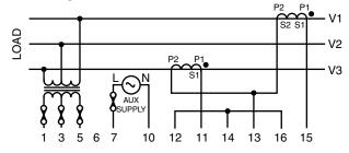
Figure 7. Electrical Connections for Single-Phase Power Circuits
