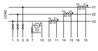
Figure 5. Electrical Connections for 3-Phase, 4-Wire Power Circuits
