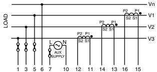
*Figure 6.* Electrical Connections for 3-Phase, 3-Wire Power Circuits using Potential Transformers
