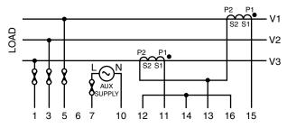
Figure 4. Electrical Connections for 3-Phase, 3-Wire Power Circuits using Three Current Transformers
